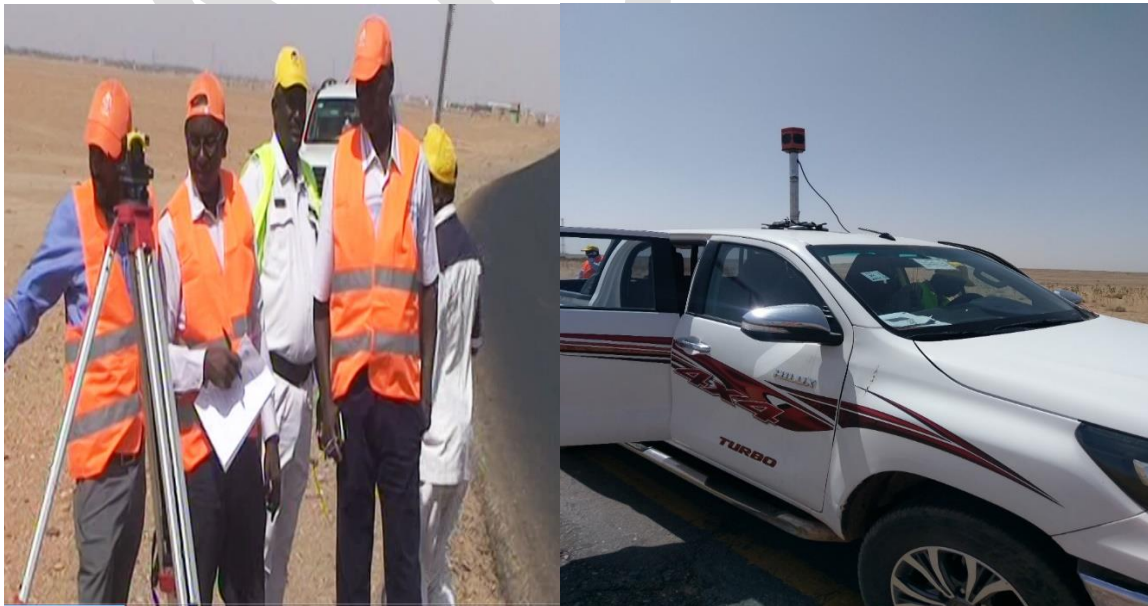
Figure 2: ADM Levelling & All – directions videoing with mounted GPS equipment's
